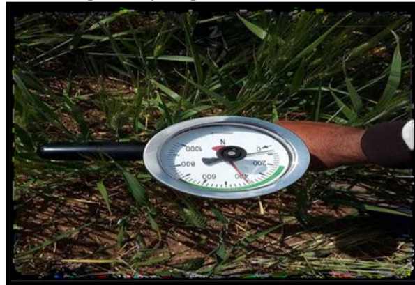
Fig. 2. Representative photo of the penetrometer measurement
